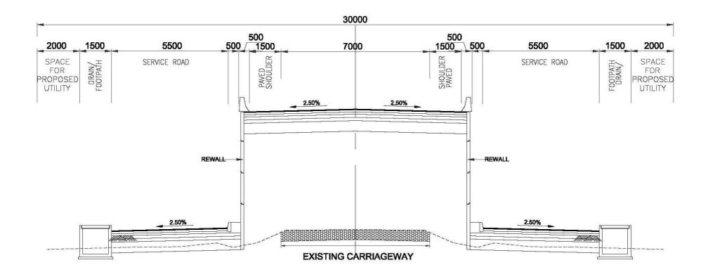
$\frac{\text{TCS - 8}}{\text{TYPICAL CROSS SECTION FOR TWO LANE VUP APPROACH WITH SERVICE ROAD}}$
